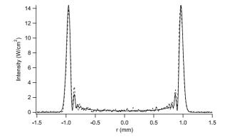
Fig. 6. Experimental (dashed line) and theoretical (full line) transverse intensity profile of the beam in  $z = 65 \text{ mm} = 2.7z_0$  after the axicon, obtained when the incident beam, with a waist  $w_i = 645 \mu \text{m}$ , crosses a convergent conical lens doublet. The convergent lens has a focal length f = 100 mm, and is located at z = -10 mm. The theoretical profile corresponds to the modelization of the axicon with a rounded vertex. Vertical scales as in Fig. 3.
