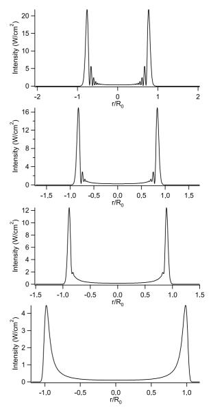
Fig. 9. Theoretical transverse intensity profile of the beam after the convergent conical lens doublet for the same parameters as in Fig. 6 for (a)  $z = 55 \text{ mm} = 2.3z_0$ , (b)  $z = 65 \text{ mm} = 2.7z_0$ , (c)  $z = 75 \text{ mm} = 3.1z_0$  and (d)  $z = 95 \text{ mm} = 4.0z_0$ . All r axes have the same absolute scale, from r = 0 mm to r = 2 mm. Vertical scales as in Fig. 3.
