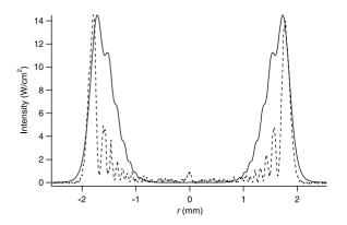
Fig. 3. Experimental (dashed line) and theoretical (full line) transverse intensity profile of the beam in z = 115 mm  $= 3.2z_0$  after the axicon, obtained when the incident beam, with a waist  $w_i = 645 \mu m$ , crosses a unique conical lens. The theoretical profile corresponds to the modelization of the axicon with a ponctual vertex. The vertical scale corresponds to the theoretical curve, when the total light power is 100 mW. Units for the experimental curve are arbitrary.
